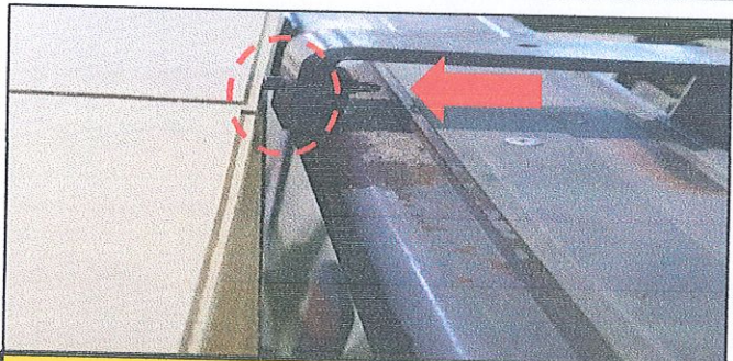
Stacking Unit Part move due to machine vibration and hit the items
